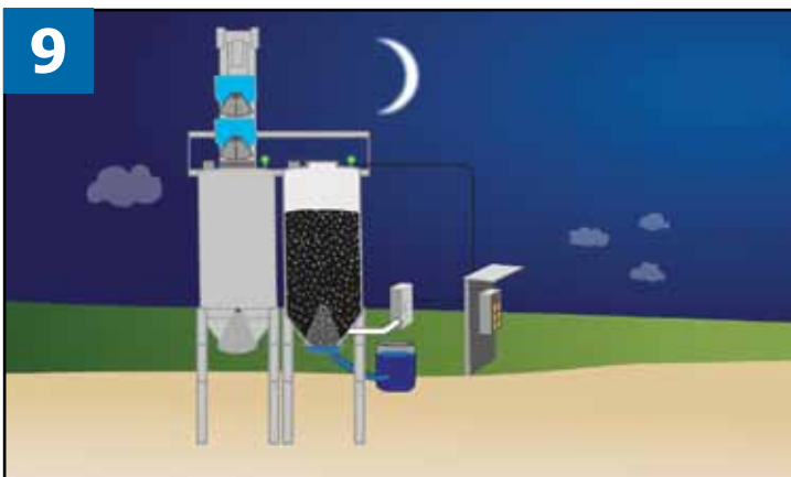
9 The asphalt is stored overnight without oxidation.
