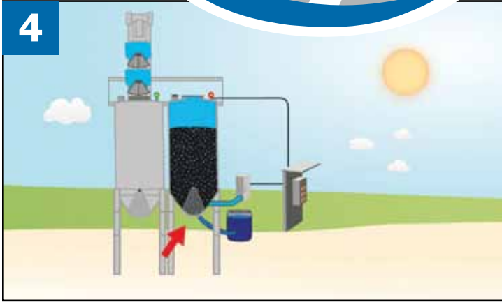
Water automatically fills the Aqua Seal™ gate.
