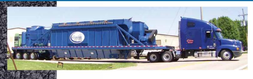
The Kleen Aire™ Baghouse is the first system to use pleated polyester cartridge filters in place of the traditional bag/cage arrangement. The pleated design of the cartridge filters provides more filtering surface area, greatly improving airflow and the ability to capture large quantities of fine airborne particulate.
