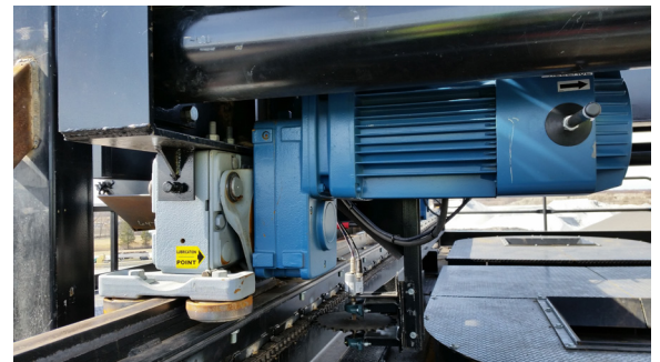
The traveling batcher drive is designed for unloading the batch into each load.
